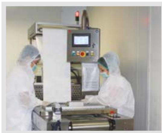
All Implance-brand products are packaged in the sterile room that fulfills sterile environment conditions according to ISO Class 7\* and air cleanliness classification standards according to ISO 14644-1.
